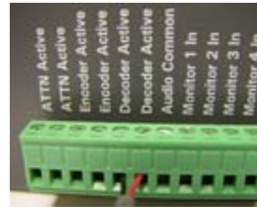
Polarity is not a factor at the Endec terminal block connection
